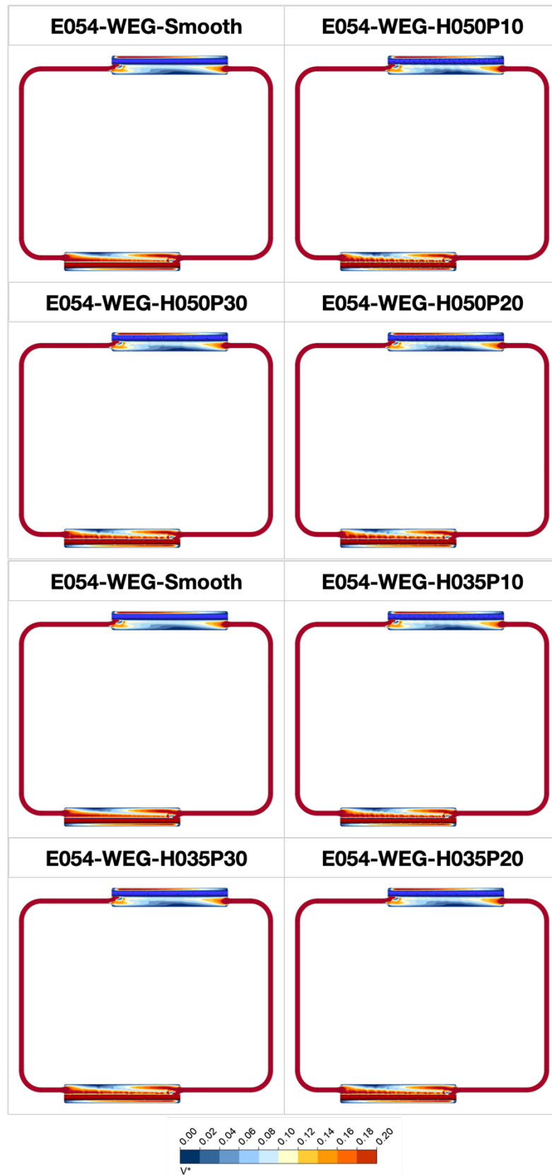
Figure 5.30: The axial V^* distribution of (a) WEG, (b) WEG+OA+SDS, (c) NF01 for different dimple heights
